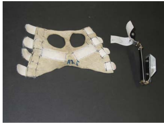
Fig. 11 Image of an example jacket and of the hinge joint which connects the jacket to the rotational joint.
