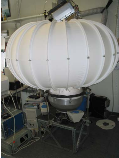
Fig. 6 Overall view of the setup with the screen lowered in working configuration. Left and right of the rack which supports the sphere (not visible), two speakers can be seen.
