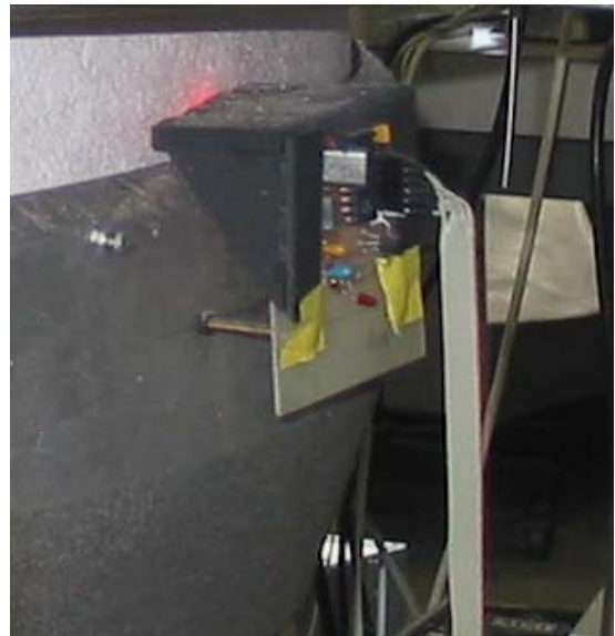
Fig. 9 Detailed view of one of the two sensors at the X position. The black cardboard provides a light shield which protects the sensor from interfering light sources.
