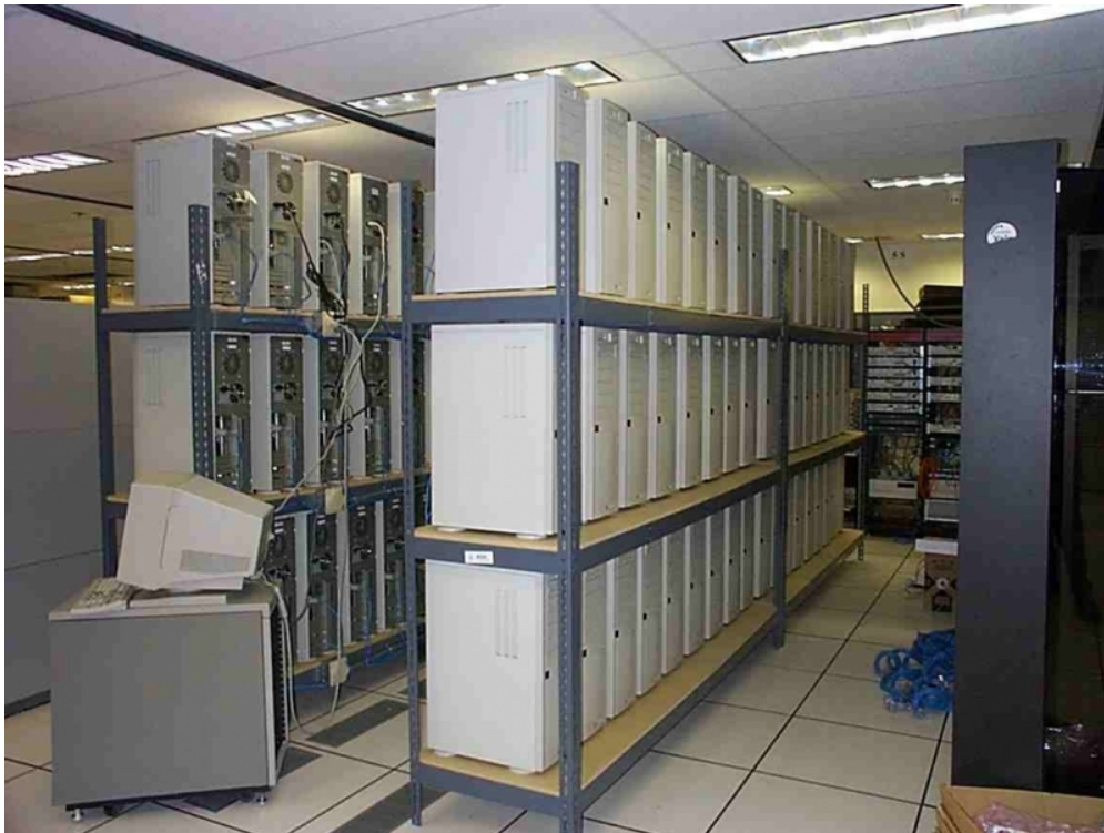
Figure 3.17: Small cluster which is built from off-the-shelf components
