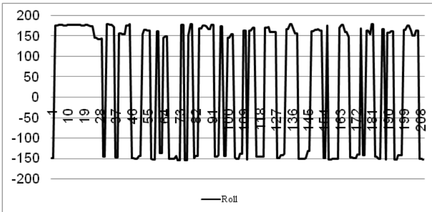
Abbildung 5.5: Typical Roll-Values occurring during a straight walk
