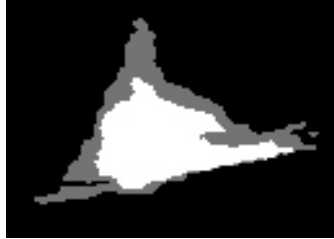
Figure 16: Depletion of the measured snow-patch from 26 July (grey, 2299 m 2 ) to 9 August (white, 1243 m 2 ) as seen by the digital camera. Note that the shape is transformed by perspective bias.
