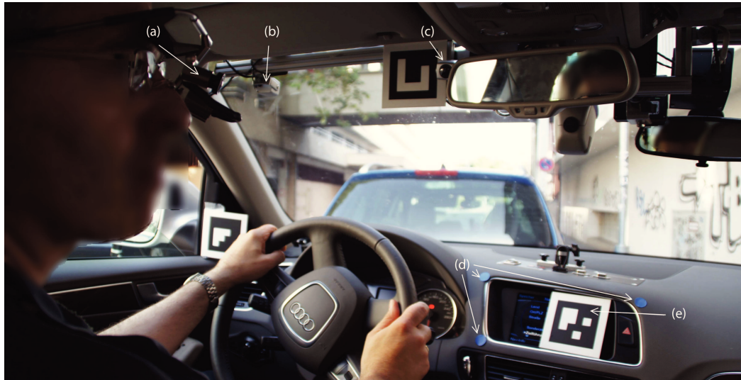
Figure 6.1: A participant wearing (a) a mobile eye-tracking head unit, (b) a camera recording the driving scene, and (c) a camera recording the driver and the car interior during the drive. (d) markers used for the calibration of the eye tracker. (e) marker used in post-processing of the raw eye-tracking data.
