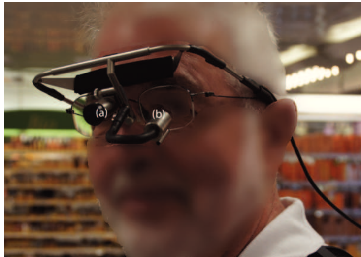
Figure 6.2: Participant wearing a Dikablis eye tracker (Ergoneers Inc., Manching, Germany). (a) field camera, (b) eye camera.
