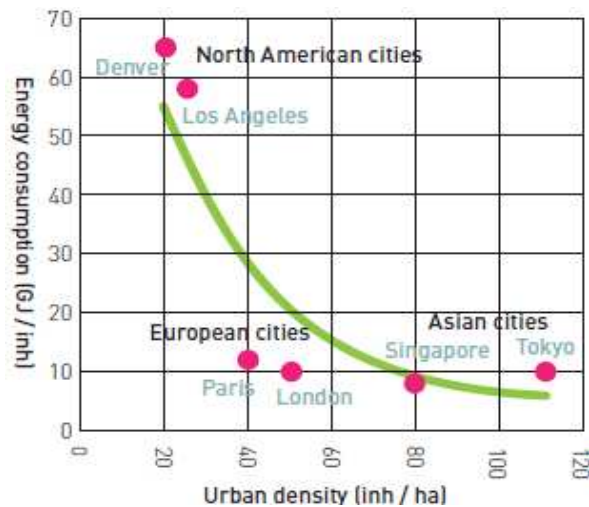
Figure 26: Energy consumption and urban density. Source: Newman & Kenworthy (1999, in: European Commission, 2010, p.6).
