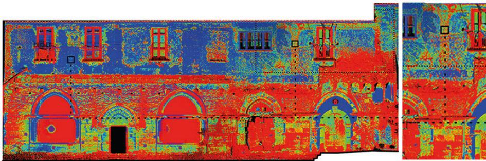
Orthophoto from laser scanning, RGB reflectance 0,24-0,37
