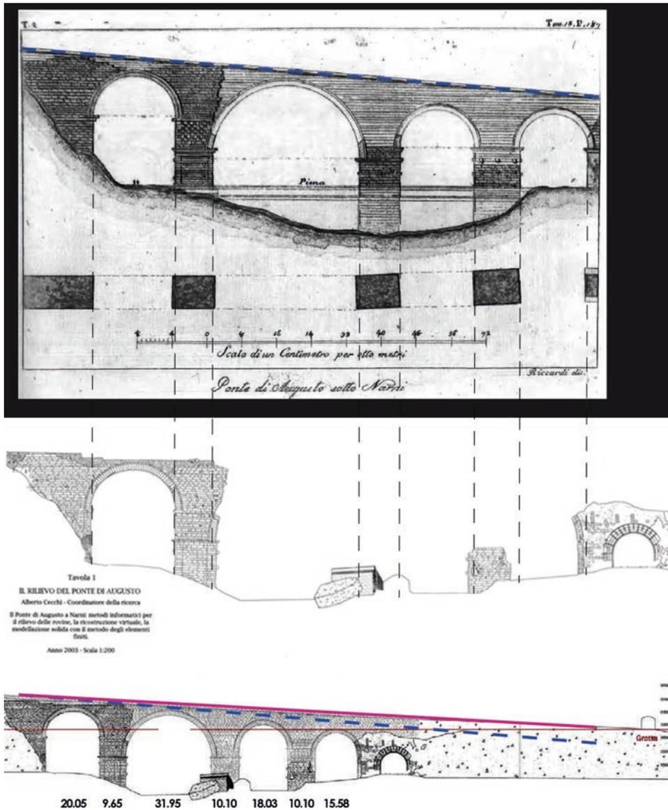
**Figure 4.** Survey and hypotheses for the reconstruction of the bridge by Eng. Giuseppe Riccardi in 1837. The differences in the springing line of the great arch, the declivity of the street and misalignment of the pillars are clearly visible (from Tattoli 2000). A comparison with Cecchi's survey. The dashed line represent the excessive slope of the road to Riccardi, compared with the slope.
