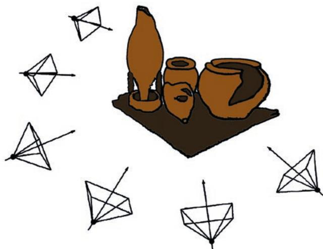
**Figure 1.** Image acquisition planning: ideally the pictures need to be taken moving around the vertical axis of the object at  $360^\circ$  for isolated objects and  $180^\circ$  for flat ones, with the camera oriented in the range of  $30^\circ / 45^\circ$ .
