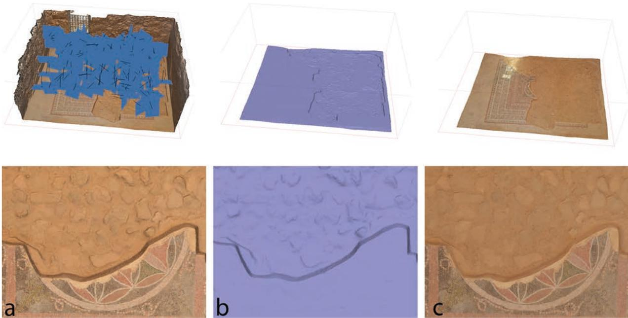
**Figure 7.** Figure shows 3d model realized through the use of Agisoft PhotoScan software. This model has a high definition texture and you can see above the details (orthorectified view) A: dense point cloud B: Mesh visualization C: Textured visualization.
