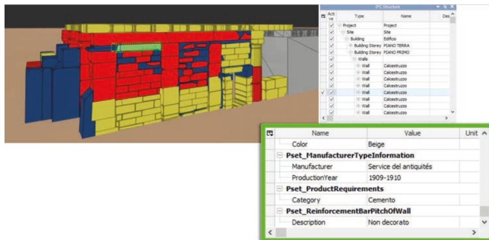
**Figure 5.** Building Information Modeling is used in order to associate additional information, such as alphanumeric data (e.g. date, material, state of degradation, management of restoration, etc.) or other files (e.g. images, archival documents, etc.) to building components. In this case, the BIM model of the Temple of Amada (Archicad 20 and IFC Viewer BIM Vision software).
