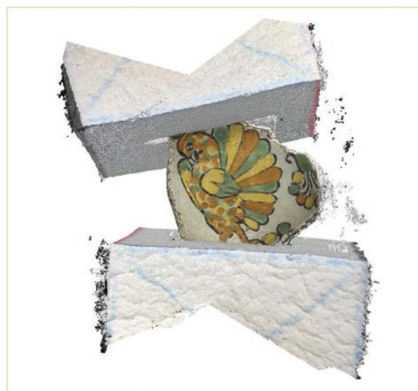
**Figure 7.** The two dense clouds of the Abó Polychrome Majolica Plate have been aligned, but the patterned blocks have not yet been deleted from the dense clouds. Note that spurious points right of the plate have not been removed in this example for illustrative purposes.
