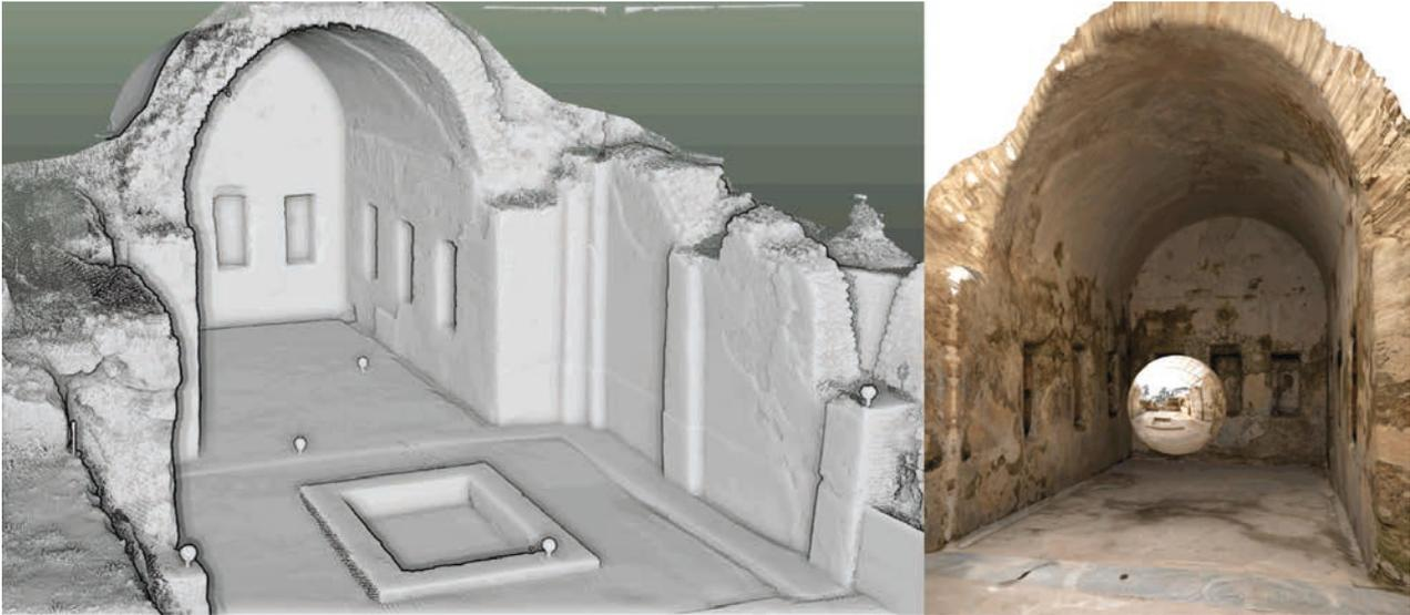
**Figure 5.** 3D elaborations from point cloud with and without texture. The texture of the 3D model was created and mapped using HDR spherical panoramas.
