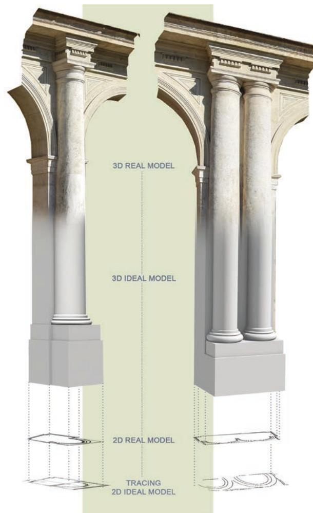
**Figure 6.** Construction of ideal 3D/2D models of the half column and the binate column. The information that could not be deduced from the worksite tracings are integrated with the images of the real elements.
