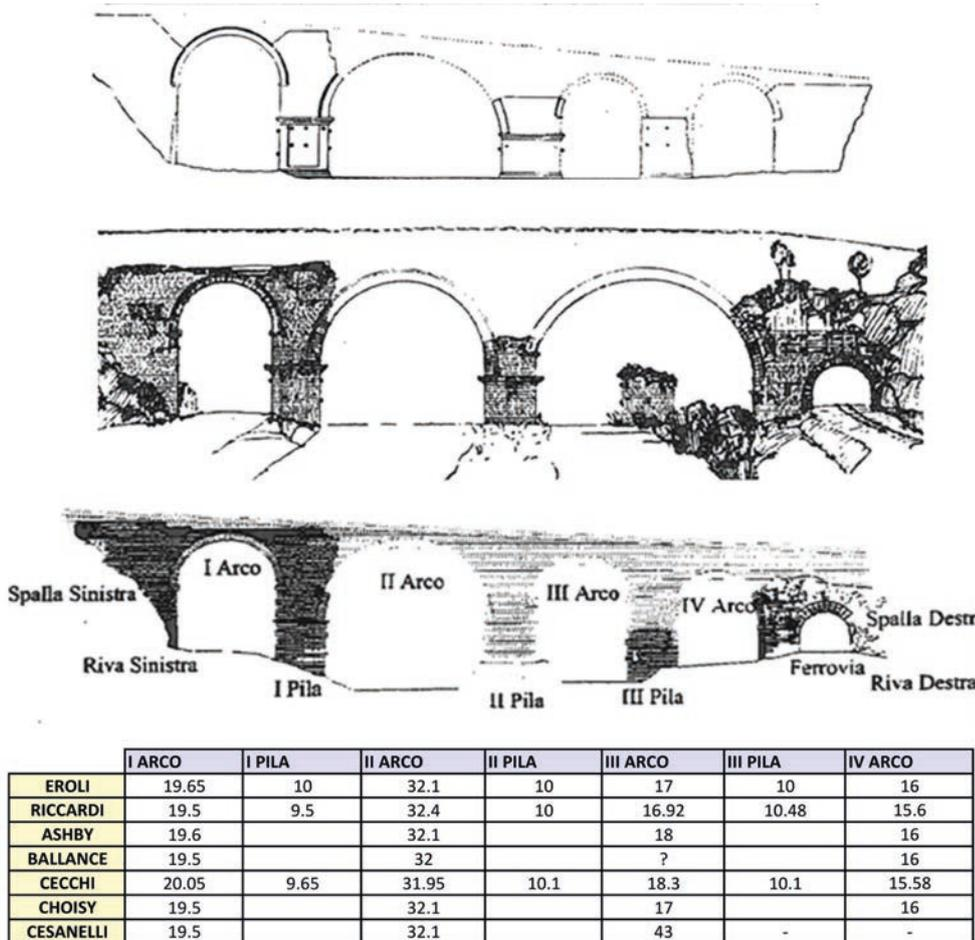
**Figure 3.** Reconstructions of the original form of the bridge made by some scholars and reported in chronological order (the measurements are in meters).
