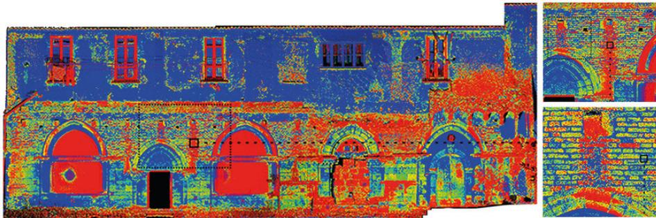
Orthophoto from laser scanning, RGB reflectance 0,22-0,30
