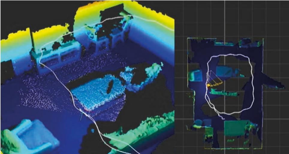
**Figure 3.** Google Tango tracks space in real-time and creates a point cloud. The numerical model is stored on the device memory, and it will update as the real environment changes.
