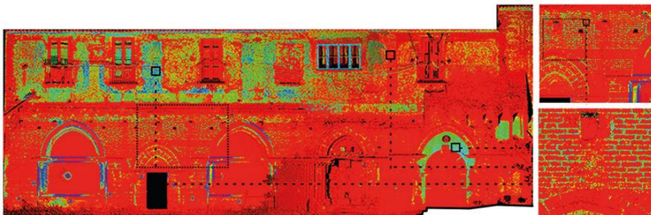
Orthophoto from laser scanning, RGB reflectance 0,35-0,48
