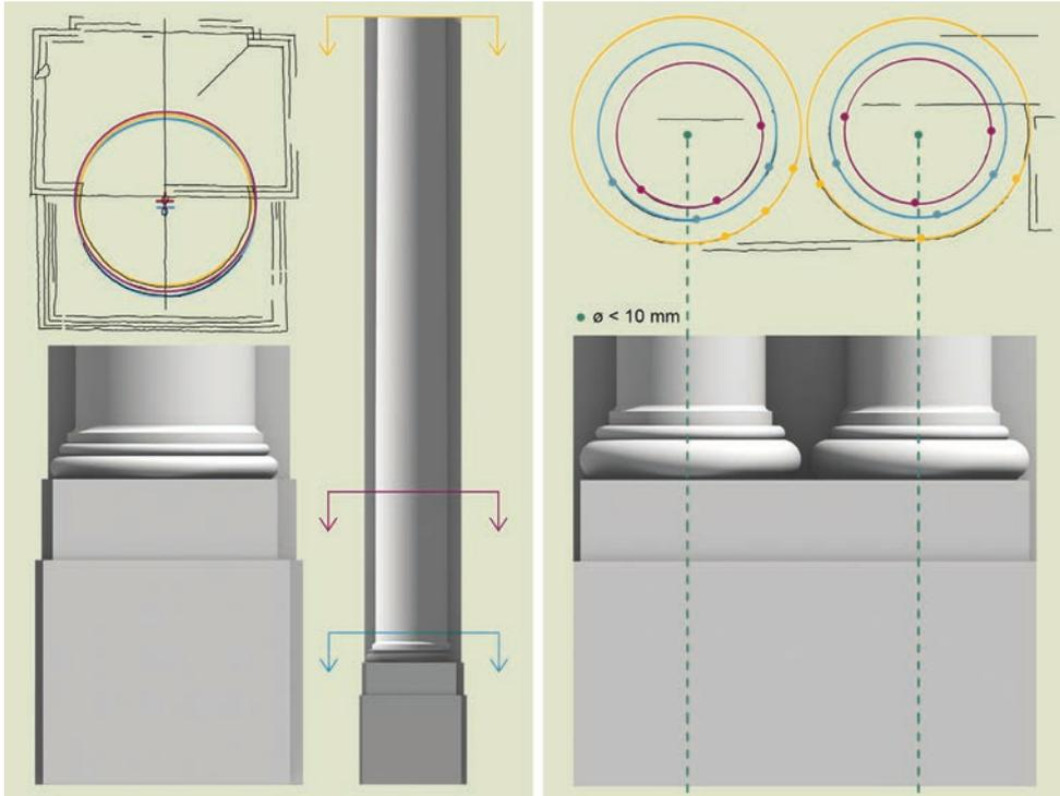
**Figure 7.** Analysis and geometric constructions of the half column and the binate column. For half column, the mouldings have been modeled on the basis of the surveying of the real element and of the tracing 5, since it is not possible to obtain enough information just from the worksite tracing 3.
