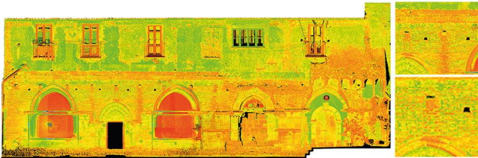
Orthophoto from laser scanning, RGB reflectance 0,18-0,23
