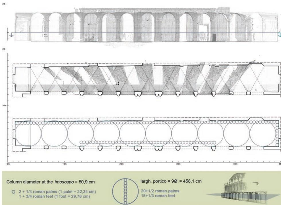
**Figure 10.** Proportion of the portico. The length, 46.31 m, corresponds to 91 modules; the width, which varies between 4.27 m on the left and 4.61 m on the right, completely match 9 modules in the central part of the façade, axis with the main portal.
