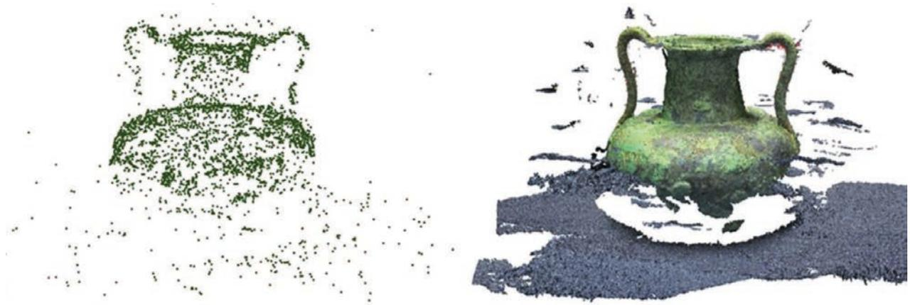
**Figure 3.** The sparse reconstruction algorithm transforms the x, y and z coordinates of common key-points in a scattered point cloud (left). The dense-matching algorithm increases the amount of data key-points giving as result a dense point cloud (right). Artefact selected in the collection of the Archaeological Museum of Amelia, Italy.
