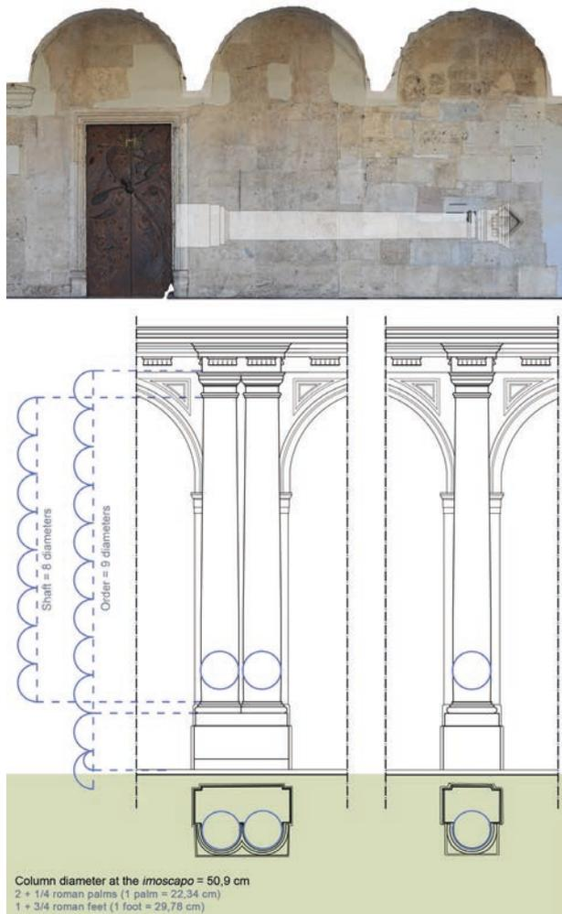
**Figure 8.** Proportion of the architectural order. The half column and the binate column. The total length of the order matches the distance between tracing 2 and the jamb of the left door of the church.
