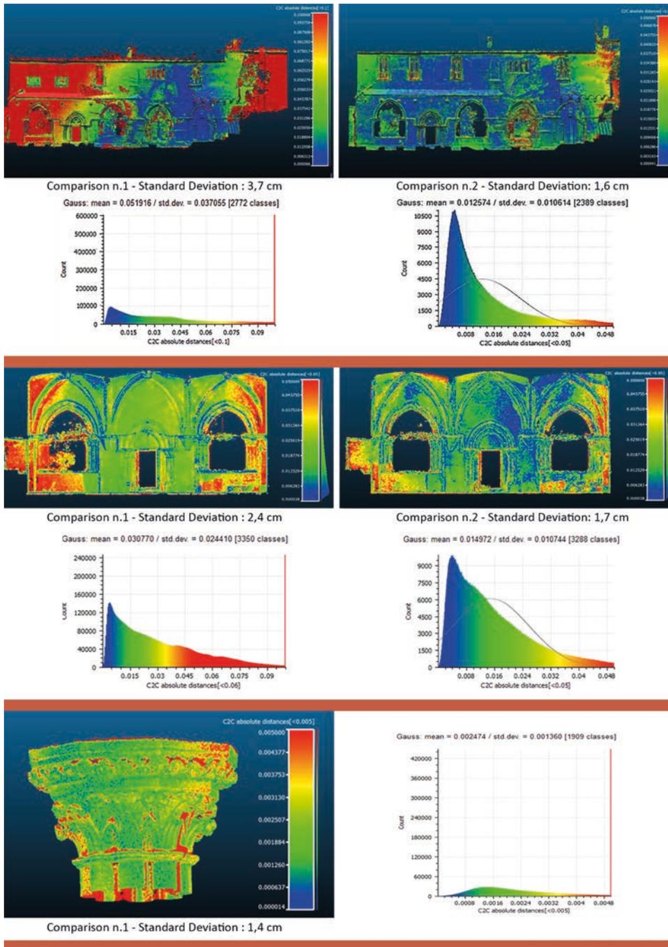
**Figure 8.** Comparison between numerical models derived from laser scanning and Structure from Motion and Image Matching, with software CloudCompare, for the three cases studies, and evidence of their deviation graphics.
