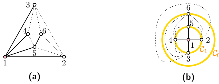
Figure 5.3: (a) The octahedral graph with a BFS-tree (bold) rooted at vertex 1 (red). (b) The corresponding ordered concentric representation.
