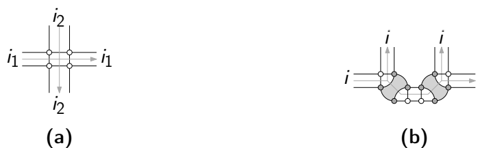
Figure 3.15: Auxiliary gadgets used by our reduction. Gray arrows show the information flow. (a) The crossing gadget lets two flows of information cross. (b) The copy gadget creates three copies of an input information.
