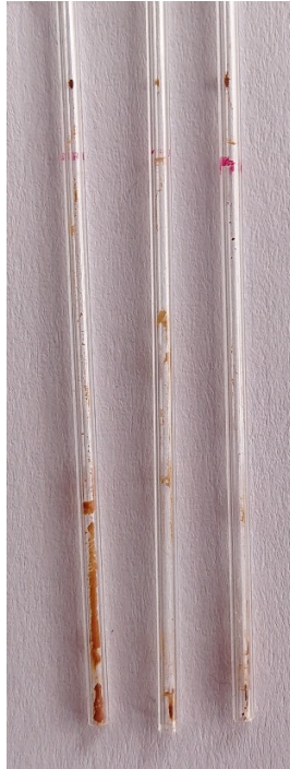
Figure S3 capillaries challenged with 1 \mu M phenylethylamine, 1 \mu M propylamine and 1 \mu M ethanol respectively. No visual response could be detected for lower concentrations.
