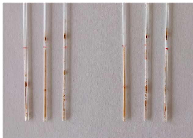
Fig. 4 shows the capillaries after reacting with ethanolamine samples (0, 25 and 75 nM) spiked in tap water and 10% serum respectively. The black/brown spots are the displaced magnetic particles after collection using a permanent magnet. For making the photos and further analysis the solution was completely withdrawn from the capillaries and the capillaries were glued to a blank paper sheet
