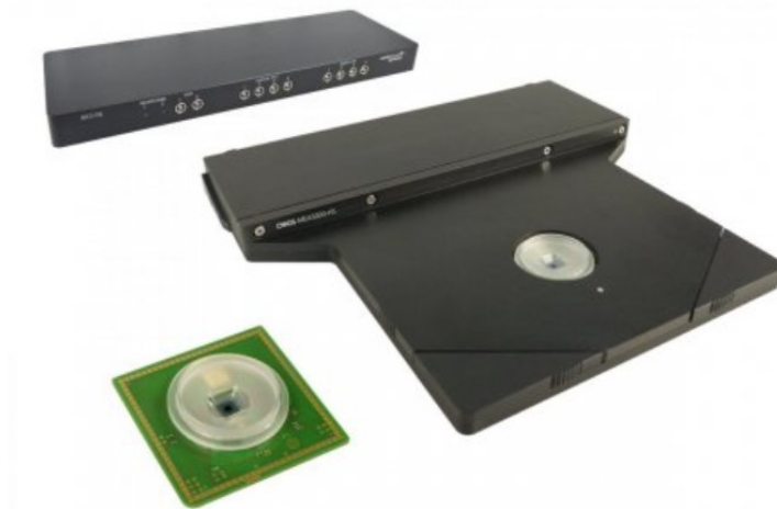
Figure 2.2: Components of CMOS 5000 system. Top: Interface-board, middle: Headstage with a mounted chip bottom: CMOS-MEA chip. Source: Multi Channel Systems MCS GmbH
