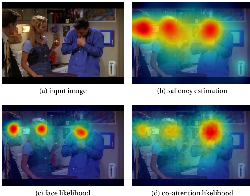
Figure C.1: Sample of a social scene in (a), and the estimated saliency map using [104] in (b). Our method, Attention Flow takes only the input image in (a) and estimate the face likelihood (c) and the co-attention likelihood (d).
