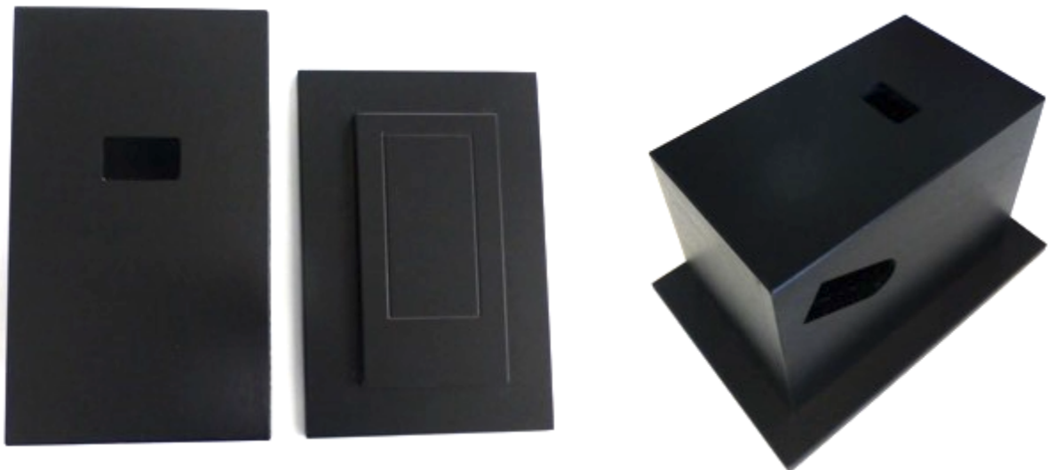
Supplemental Figure S5: TLC imaging box from Pidinger Werkstätten.
