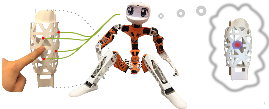
Figure 2.1: Overview of the method: Inferring single contact haptic information from a few sensors. We modify the shin part of a humanoid robot to validate our proposed idea.
