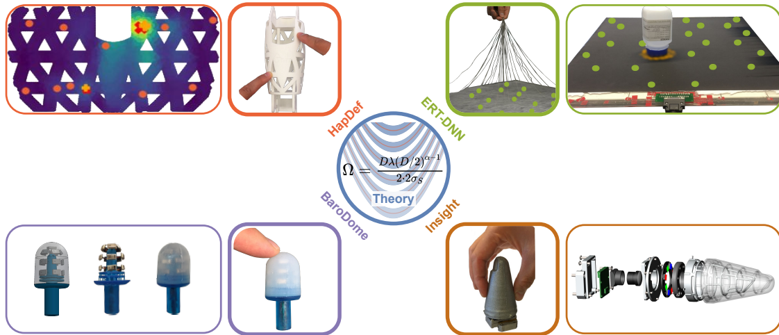
Figure 1.2: Thesis contribution overview. Red boxes describe the project HapDef . When two fingers contact the 3D curved skeleton, the deformation is inferred from ten sensor elements (red dots), shown as an unfolded 2D plan in terms of a color map. The contact locations and forces are then extracted accordingly. Red crosses and yellow pluses are ground truths and predictions, respectively, with variant sizes indicating different forces. Green boxes describe the project ERT-DNN . A few flexible and conductive sewing wires (green dots) are sewed on the conductive fabric. There is a conductivity change upon object contacting, as shown in the orange shade around the contact area. A machine learning model is built to infer the contact locations and forces for multiple contacts from the raw measurements. Purple boxes show the project BaroDome . A few barometers are sparsely embedded in a full soft elastomer to measure internal pressure changes. A machine learning pipeline is established to predict contact information. Brown boxes describe the project of Insight . A high-resolution camera is enclosed to view a soft shell from within, and machine learning is used to infer the force distributions over the outer sensing surface. The blue circle belongs to the project Theory . The theory explains the super-resolution working mechanisms. The capital \Omega is the super-resolution factor.
