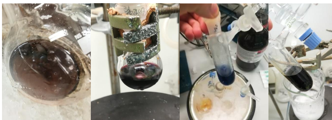
Figure 4.3. Oxygenated manganese reagent solutions from left to right: 2-Methylpropyl-( 143j ), iso -propyl ( 143c ), tert -butyl ( 143f ) and benzyl ( 143h ) manganese halide (colors from left to right: brown-purple, wine red, ink blue, black-green).
