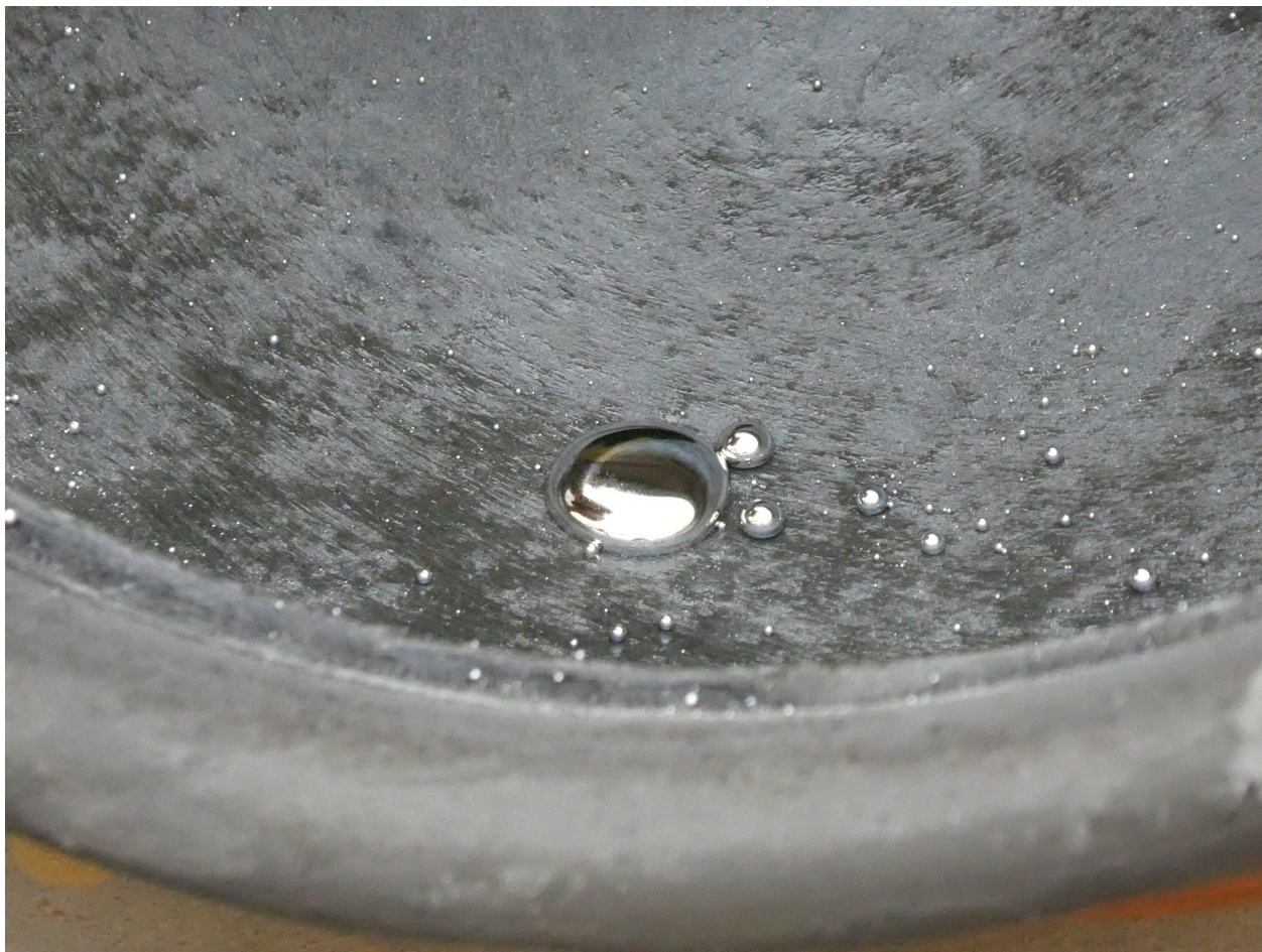
Fig. 2. Liquid elemental mercury in a clay vessel after extraction from mercury sulphide through calcination (Photo by Roman Sieler).
