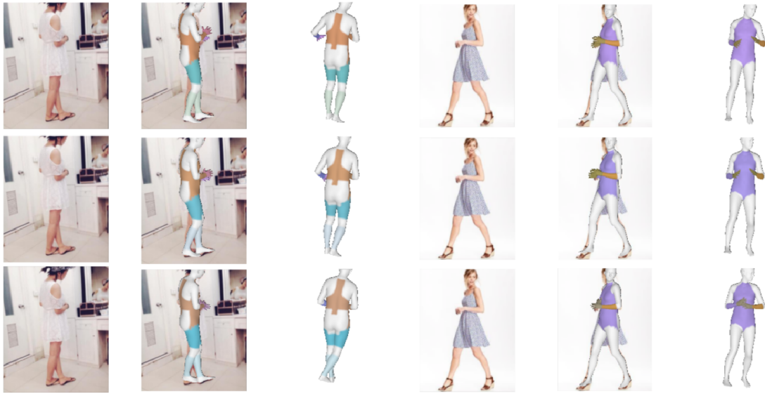
Figure 2.12: Impact of discrete self-contact labels in human pose estimation. Body parts labeled in contact are shown in the same color. First row shows an initial SPIN estimate, second row the SMPLify fit, third row the SMPLify-DC fit after 20 iterations.
