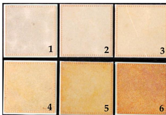
Figure 4.1: Direct bonded copper Curamik®Power substrates. (1) is an example of sample type 1, (2) sample type 2, (3) sample type 3, (4) sample type 4, (5) sample type 5 and (6) sample type 6.
