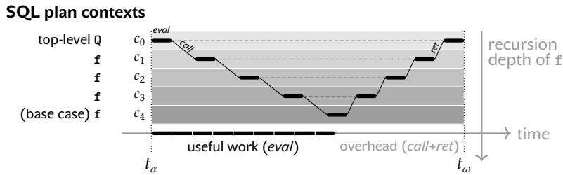
Figure 8.3.: Nested plan contexts built to evaluate a top-level SQL query Q that contains a call to a linear-recursive UDF f . Overall evaluation time for Q is t_\omega - t_\alpha .
