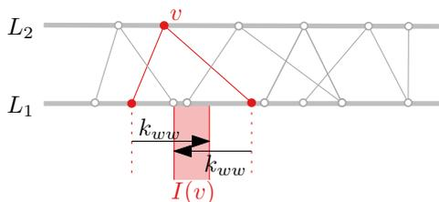
Figure 3.20: Showing the construction of an interval  $I(v)$ . While very similar to the interval construction in 3.1, the initial intervals differ significantly.
