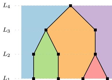
Figure 5.7: The areas corresponding to mutual ideal positions are marked by color for this instance. Specifically for any vertex  $v$  at a position of a given area, the ideal position of a child of  $v$  is within the same area on the layer below. We can see, that these areas closely resemble faces, however they are not closed at the leaf layer.
