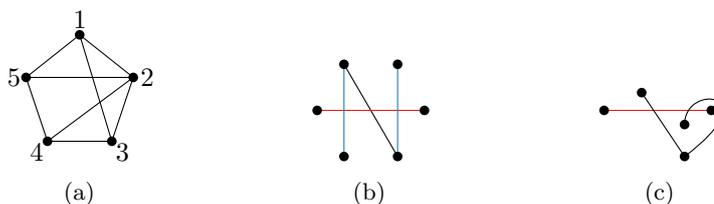
Figure 2.13: (a) A fanplanar drawing, both edges crossing  $(1, 3)$  share a common vertex 2. (b) A forbidden configuration of fanplanar drawings, where both blue edges are crossed by the red edge, but they are not incident to a common vertex. (c) Another forbidden configuration of fanplanar drawings, the red edge is crossed by two edges with a common vertex, but with different orientations.
