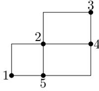
Figure 2.7: A planar orthogonal drawing of graph  $G = (\{1, 2, 3, 4, 5\}, \{(1, 2), (2, 3), (3, 4), (4, 5), (5, 1), (2, 5), (2, 4)\})$ .
