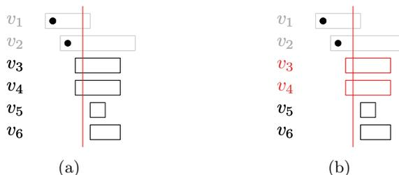
Figure 3.7: Showing the sweep-line (a) before and (b) after two start events adding  $I(v_3)$  and  $I(v_4)$  as active intervals.
