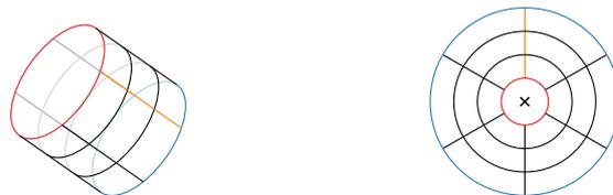
Figure 7.1: A 4 by 6 grid projected to (a) a cylinder,(b) the plane, where it is drawn as an ortho-radial grid.
