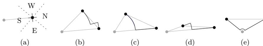
Figure 7.11: Edge representations with **port by angle** strategy: (a) The sectors indicating which port to use. The center point is shown in gray (b)  $e$  uses the east port at  $v$  and the west port at  $w$ . (c)  $e$  uses the east port at  $v$  and the south port at  $w$ . (d)  $e$  uses the north port at  $v$  and the west port at  $w$ . (e)  $e$  uses the south port at both  $v$  and  $w$ .
