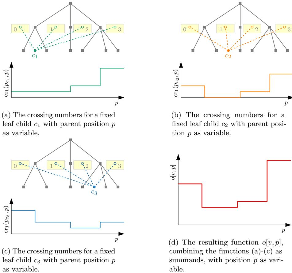
Figure 5.8: An example, depicting how  $o[v, p]$  corresponds to a unimodal function with  $p$  as the variable, which is the sum of multiple unimodal functions.
