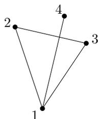
Figure 2.1: A pictorial representation of a graph  $G = (V, E)$  with  $V = \{1, 2, 3, 4\}$  and  $E = \{(1, 2), (2, 3), (1, 3), (1, 4)\}$ . Vertices are represented as dots and edges as lines connecting adjacent vertices.
