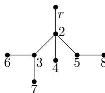
Figure 2.2: A rooted tree consisting of 8 vertices and 7 edges. The vertices 4, 6, 7 and 8 are leaves. Root  $r$  is not a leaf.
