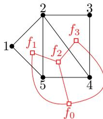
Figure 2.6: Graph  $G = (\{1, 2, 3, 4, 5\}, \{(1, 2), (2, 3), (3, 4), (4, 5), (5, 1), (2, 5), (2, 4)\})$  with dual graph  $G^* = (\{f_0, f_1, f_2, f_3\}, \{(f_1, f_2), (f_2, f_3), (f_3, f_0), (f_0, f_1), (f_0, f_2)\})$  shown in red. Face  $f_0$  is the outer face.
