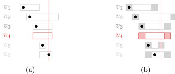
Figure 3.10: Showing the sweep-line (a) before an end event for  $v_4$  and (b) after an end event for  $v_4$ . The temporary Window Width  $k_{ww}$  is incremented as  $I(v_4)$  is still active. Observe that all intervals are increased by 1 in each direction and the assignments which already have been made are shifted by 1 to the left. Thus the current position becomes free.
