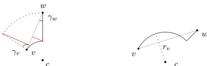
(a) Schematic showing the distances between bend points and straight line segment depending on whether  $v$  or  $w$  is incident to the circular segment. The distance is shown in red.
