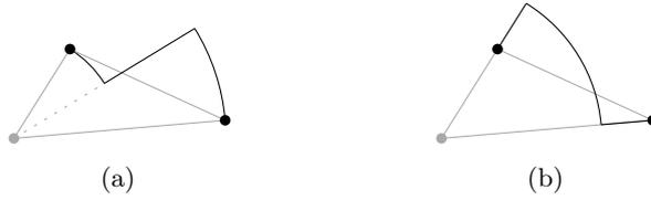
Figure 7.9: Edge representations with **uniform steps**: (a) circular step (b) spoke step.
