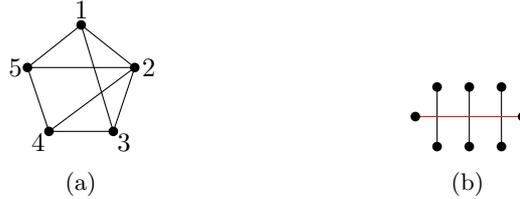
Figure 2.11: (a) A 2-planar drawing, where the edge  $(1, 3)$  has the maximum of two intersections. (b) An instance showing the forbidden configuration of 2-planar drawings, where the red edge has 3 crossings.
