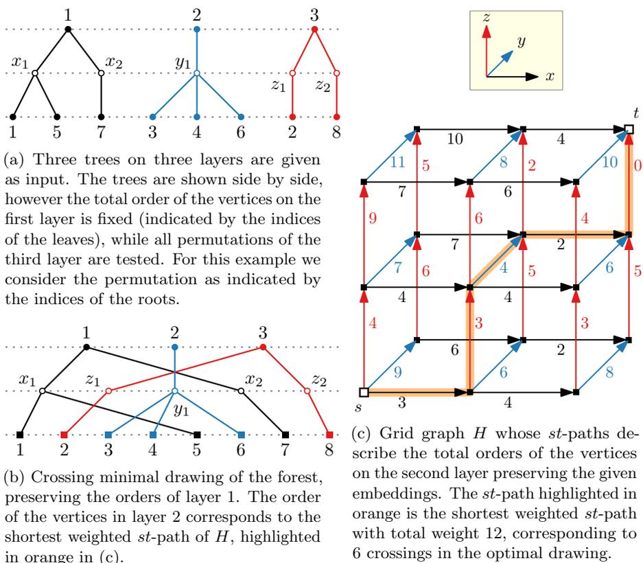
Figure 6.2: Reducing the problem of finding a crossing minimal drawing on three layers to a shortest-path problem in a weighted  $k$ -dimensional grid graph.
