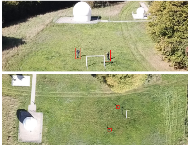
Figure 3.1: Example images of the data set POG, showing the same scenery taken from different perspectives (top: 10m, 10°, bottom: 100m, 90°).
