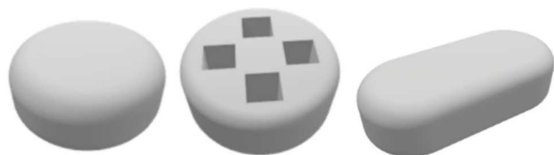
Fig. 1. .stl files of tablets printed; fltr: round tablet with rounded edges, round tablet with rounded edges and pores, exemplary oblong shaped tablet used in dosage trials.
