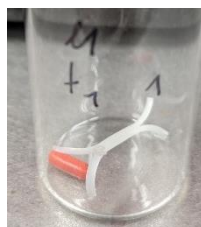
Figure 3 PVA filament stored in ibuprofen-saturated methanolic solution
