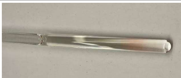
Figure D.10: Red coloring of a solution of TIPS4Hep in \text{CCl}_4 after attempted fluorescence spectroscopy. Only the part where the excitation light beam hit the sample a red coloration is visible.
