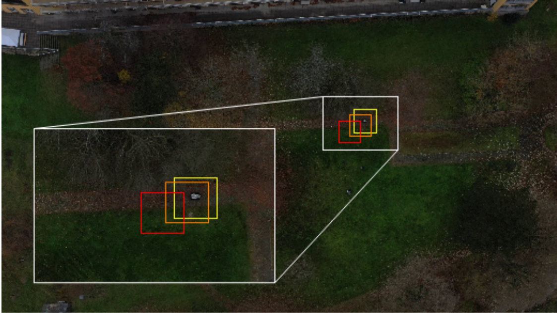
Figure 4.13: Example calibration procedure: We know the GPS position of the robot. Projecting the GPS location to image space yields the red bounding box. Taking the distance to the yellow box as loss, we optimize the gimbal pitch angle, heading angle, and GPS longitude and latitude parameter offsets that might have occurred, leading to a better calibrated metadata measurement. After calibration across several frames from different viewpoints, we obtain the orange box.
