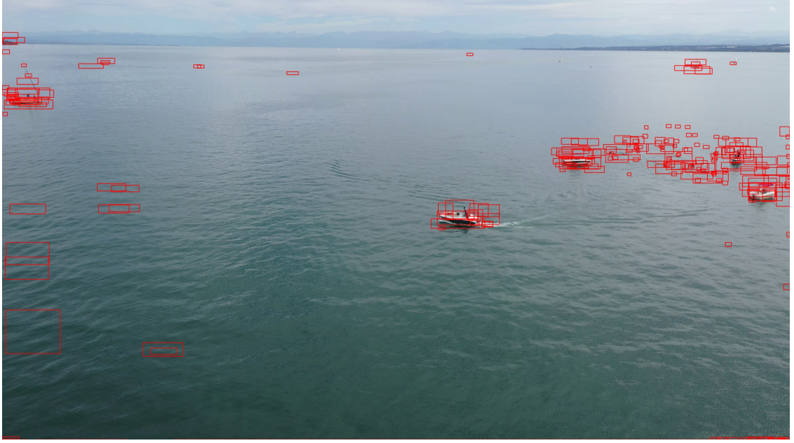
Figure 4.7: Before NMS, there are many low-confidence detections, but they cluster around actual objects. Ignoring the confidence, these detections would yield a recall value of one. For visualization, only one-colored boxes.
