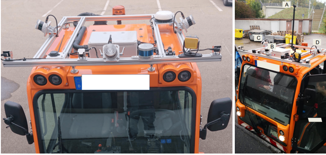
Figure 3.2: Sensor setup on the data collection vehicle. Ouster lidar sensors are positioned at the front, right, and left (B, C, D). The 360° camera is mounted at A.
