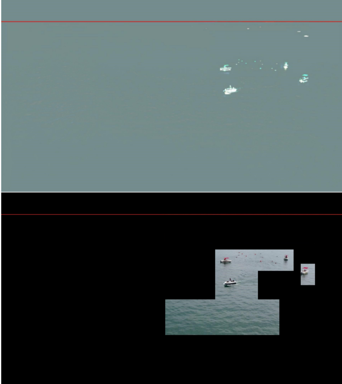
Figure 4.11: Difference anomaly map aggregated in 3D space over several frames (top) and resulting regions of interested (bottom).
