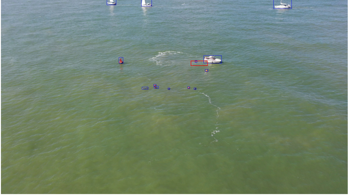
Figure 4.4: Blue boxes are true positive detections, the red box is a false positive swimmer detection that was successfully filtered out by analyzing the distance-size relation.
