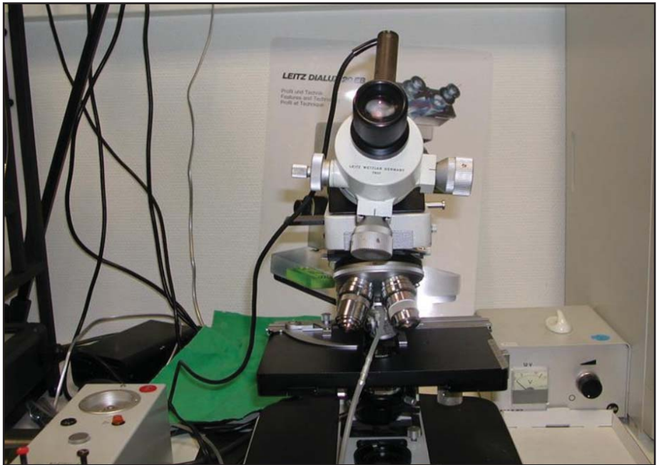
Fig. 7. The Vickers microhardness-measuring device used in the present study (Leitz, Frankfurt)
