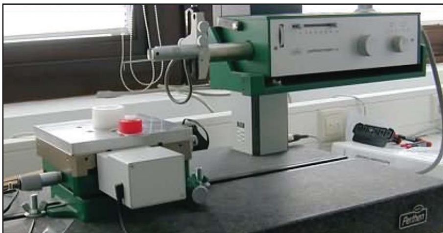
Fig. 6. The profilometer used in the present study (Perthometer 3D, Mahr, Goettingen).
