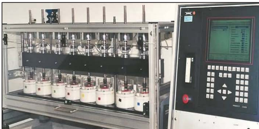
Fig. 9. Picture of the chewing simulator used in the present study (Willytec, Munich).
