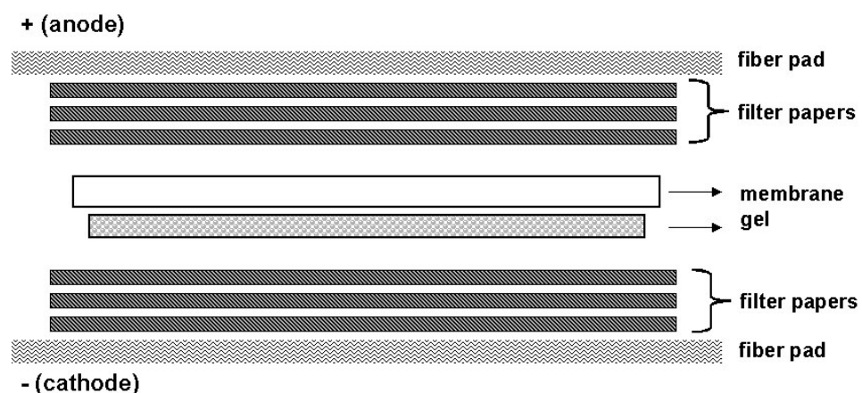
Figure 9. Schematic representation of the membrane-gel sandwich assembly for the electrophoretic transfer of proteins from the gel to the nitrocellulose membrane.
