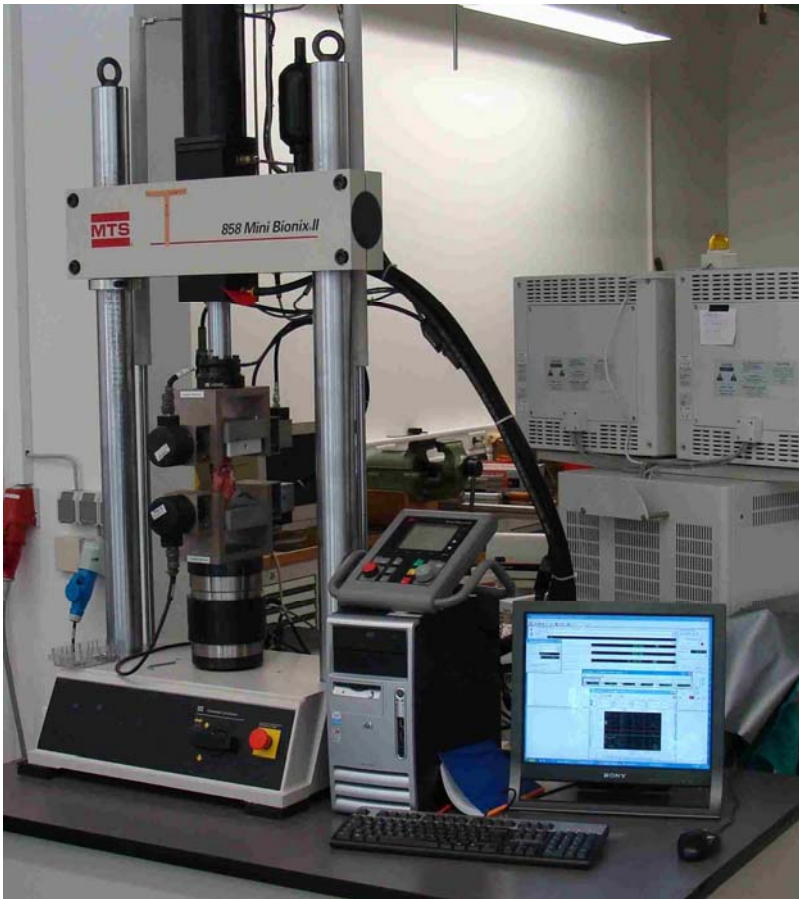
Fig.13: The friction apparatus system consists of a capture computer and a MTS machine, which includes an upper spine and a lower spine mounting mechanism.
