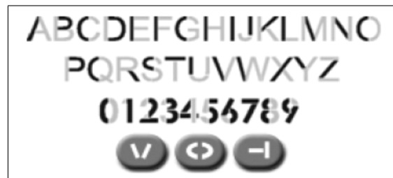
Figure 2.5: The three keys of the Uniglyph ambiguous keyboard, representing character primitives (cf. Belatar & Poirier, 2007)
