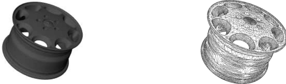
Figure 2.17: Car felly in a distance of 0.5 m from the observer with image size 150x150 and the corresponding wireframes with 14,489 points and 25,661 triangles.
