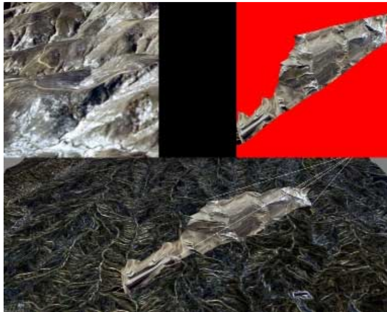
Figure 1.22: Conversion of central projected aerial photos to orthographic, geo-coded images, see also [39]. On the upper left, the original image is shown, which is projected in the lower image with a central projection on a digital elevation model (DEM). From this, the orthographic, geo-coded image on the upper right is produced with an orthographic projection.
