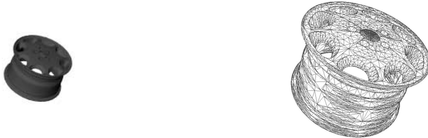
Figure 2.18: Car felly in a distance of 0.5 m from the observer with image size 81x81 and the corresponding wireframes with 7,344 points and 12,606 triangles.
