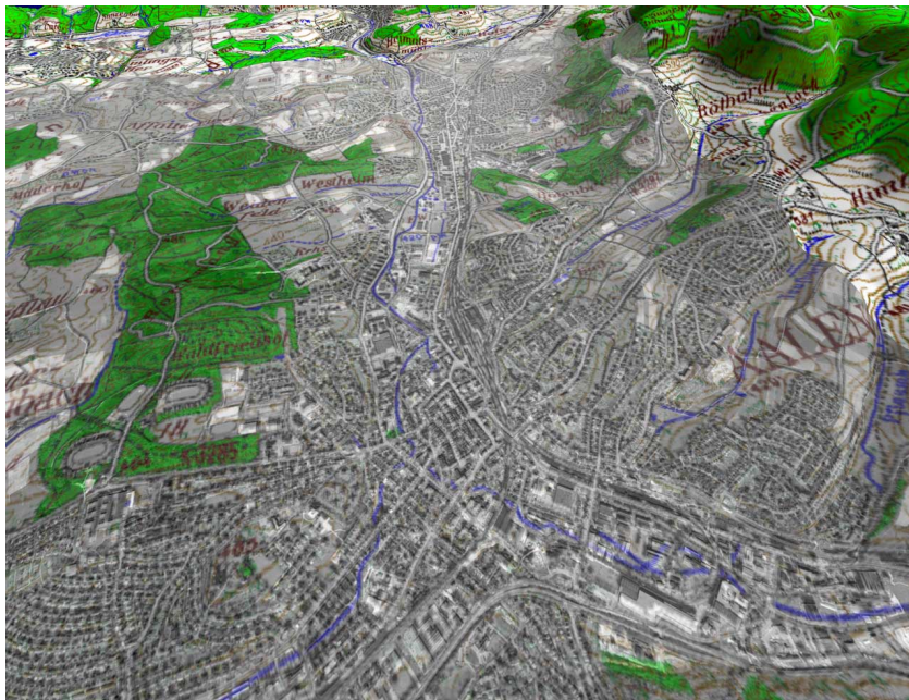
Figure 5.12: Topographic map with superimposed orthographic photograph. The orthographic photo is blended with the map below.
