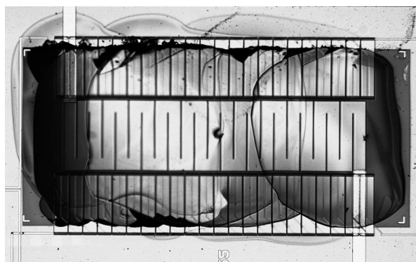
Fig. 4.3.6.4: PEUT layer on a cracked , sensing membrane of a calorimetric sensor (dimensions 750 \times 1500 \mu\text{m} ).
