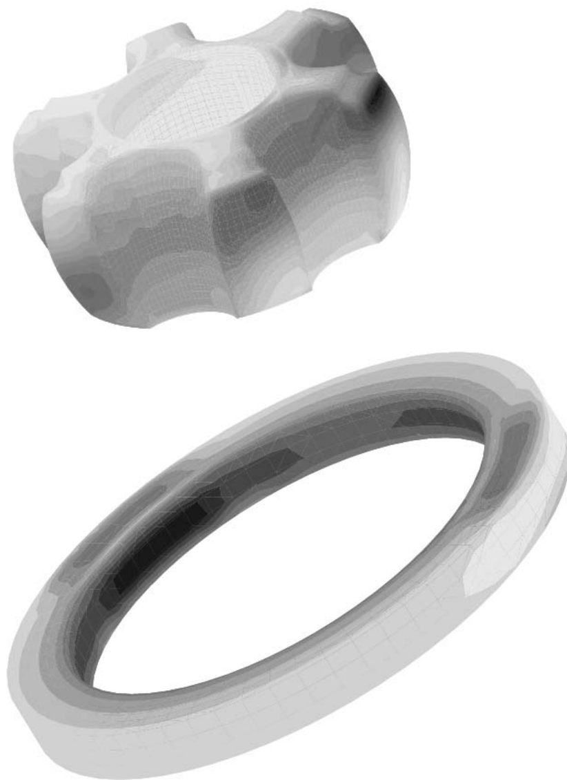
Figure 7.3: Current in workpiece and inductor
