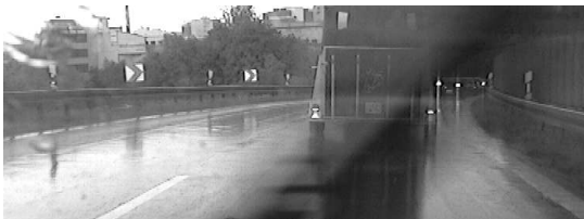
Figure 2.6: Temporary Loss of an Image: Due to the windshield wiper passing a camera, an image frame is lost for processing.
