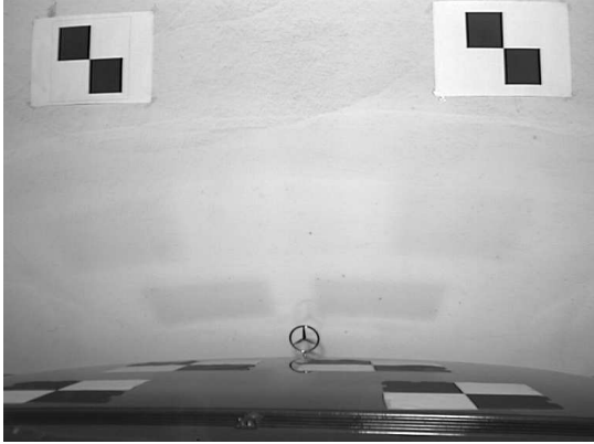
Figure 8.3: Setup to Determine the Influence of Vibrations: Patterns are attached to the wall and to the hood. Note that the pattern on the hood are not reflections but attached markers.
