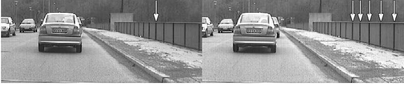
Figure 2.4: A Multiple Matching Hypotheses Situation: An image pair exhibiting a multiple matching hypotheses situation. The features of the pillar marked in the left image are found in the right image several times. Choosing the wrong match leads to a wrong environment representation. A feature matching with distance information are shown in Fig. 2.5
