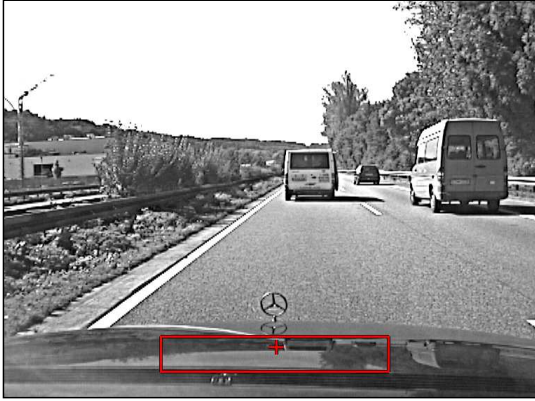
Figure 8.9: A Typical Traffic Scene in a Vehicle Following Application. The box marks the region of interest which is reconstructed. The cross is the location of the tangential point chosen for the Comparison-of-Lines method.
