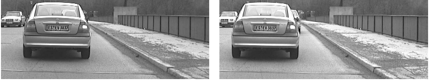
Figure 1.1: A Stereo-Camera Image-Pair with Repetitive Patterns: The pillars of the guardrail are repetitive patterns.
