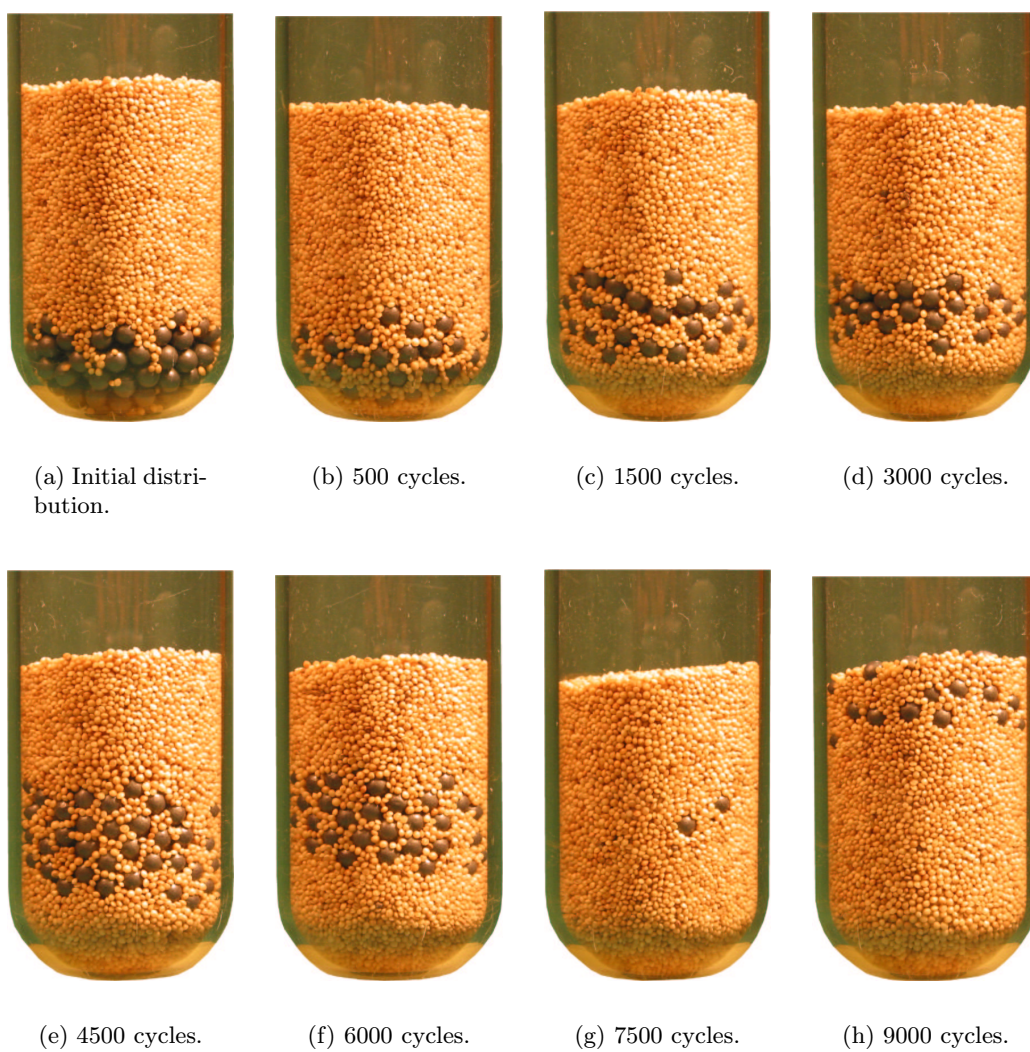
Figure 9.3: Vibration of a mixture of amaranth and lead balls. The Brazil nut effect dominates and drives the lead balls to the top in spite of their high specific weight.
