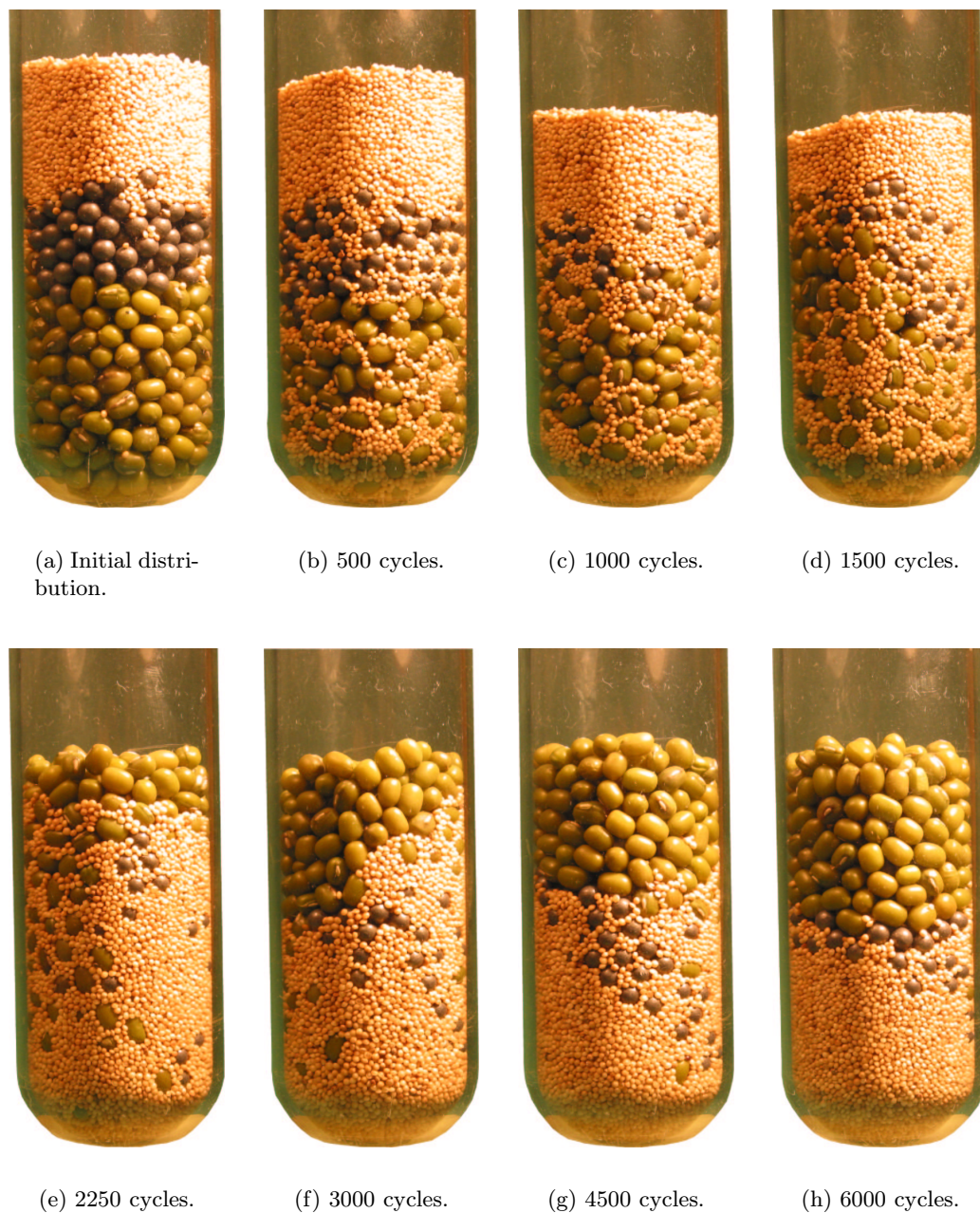
Figure 9.4: Vibration of a mixture of green gram, amaranth and lead balls. Again, the large seeds of green gram come to rest on top, while amaranth forms the bottom layer. In spite of their high specific weight, the lead balls of intermediate size form the middle layer.
