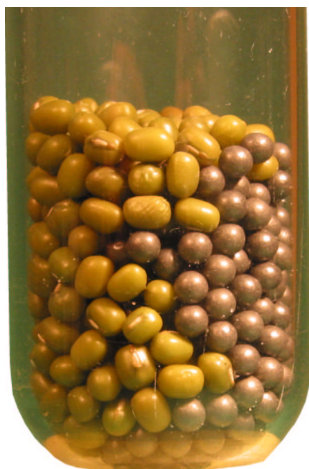
(a) Convection roll in a shaken mixture of green gram seeds and lead balls. The snapshot shows horizontal segregation with green gram on the left and lead balls on the right.
