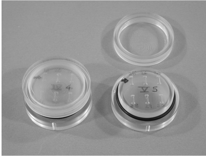
Figure 1. A detailed view of the PMMA container used for the measurements. It can hold up to six TL detectors. The diameter of the container is 30 mm.
