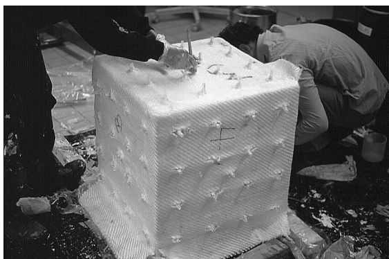
Figure 2.3 Photograph of the resin coating of the sandstone block [from LEVEN ET AL., 2004].
