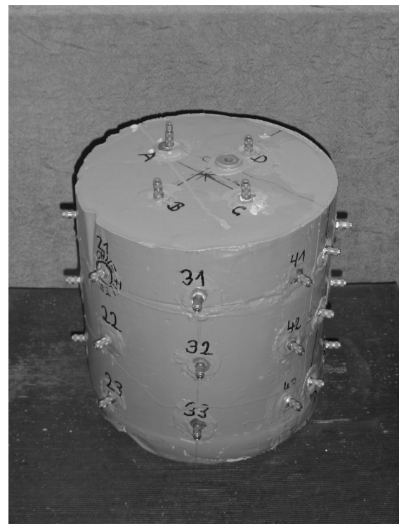
Figure 4.2 Photograph of the investigated gas saturated fractured sandstone cylinder after the preparation for the experiments.
