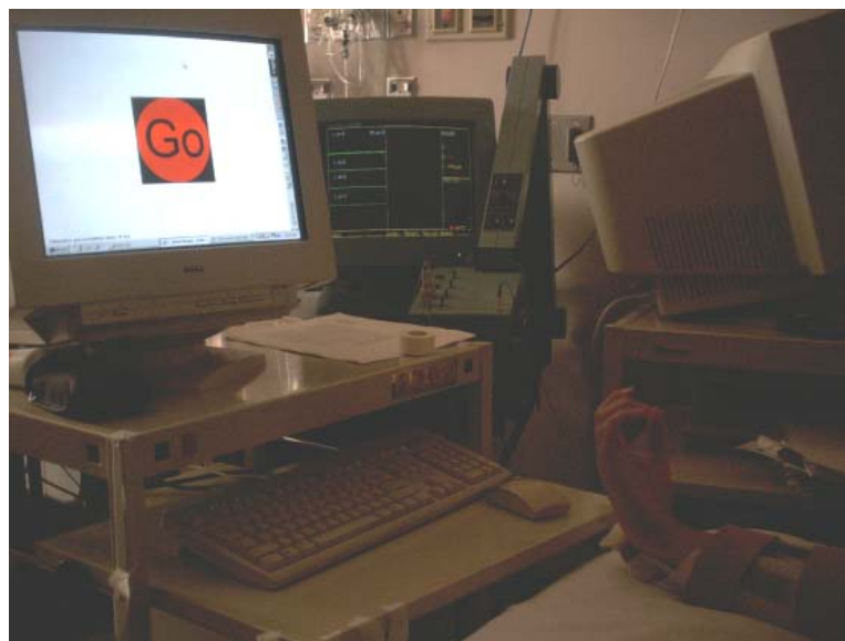
Fig. II.4: Wrist flexion was performed after a GO signal on the screen. Reaction time was measured using an electromyogram.
