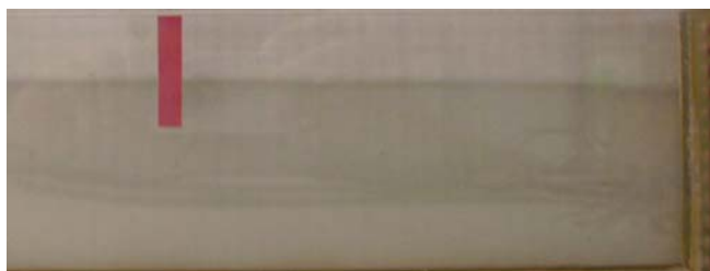
Figure 5.2 Tank used in the experiment (the red tape is the oxygen sensitive foil which is glued on the inner wall of the tank)
