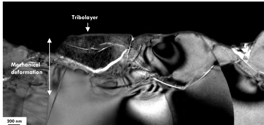
b) Without external cooling: smooth part (TEM bright field)
