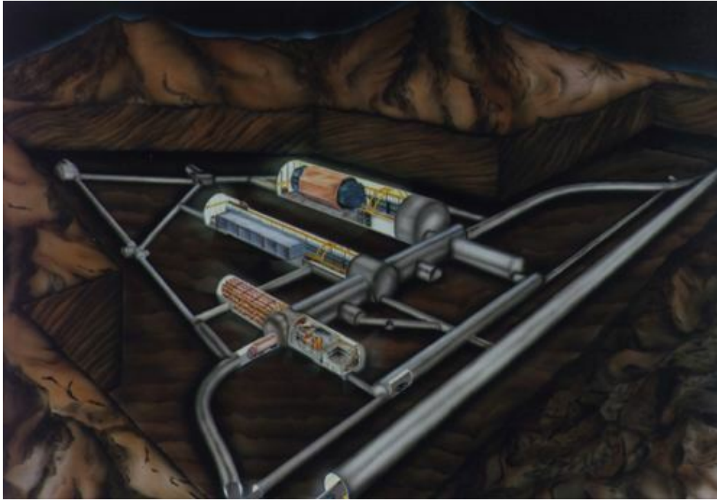
Figure 5.1: The CRESST experiment is located in the Italian national laboratory under the Gran Sasso mountain (LNGS). The experimental setup is in the smallest cave, cave A, which is the most front one in the picture [42]. All caves can be reached by car via a bypass of the Rome–Teramo highway in the Gran Sasso tunnel. The whole laboratory is shielded by the mountain against cosmic radiation.
