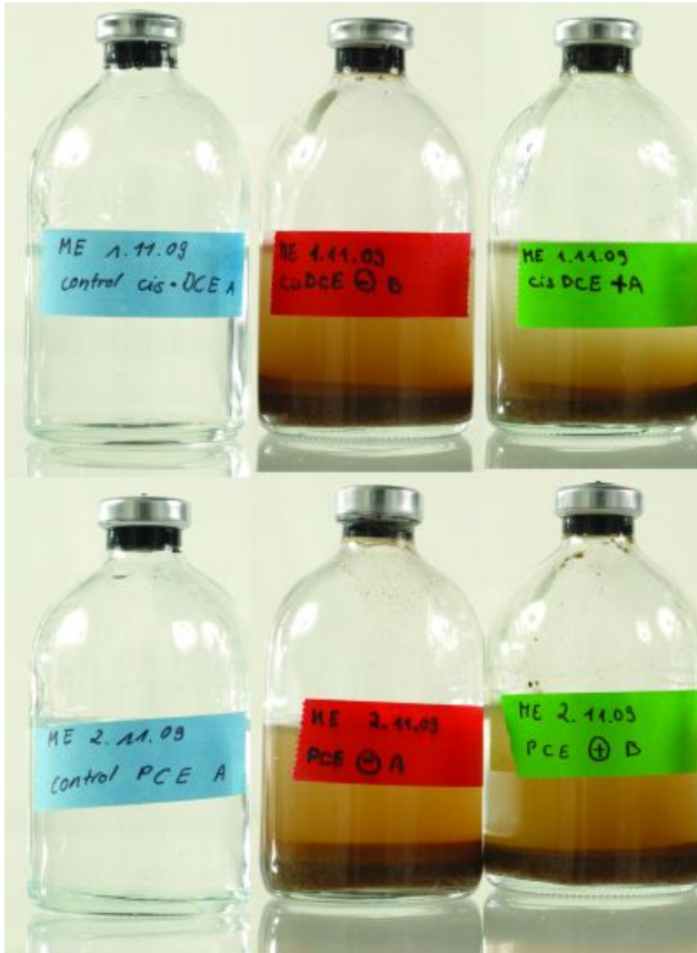
Figure 2: Microcosms spiked with cisDCE (top row) or PCE (bottom row). The left bottles display (glass and stopper) sorption control setups. Setups in the center contain sterilized KasinI.1 sediment and setups in the right are microbially active.
