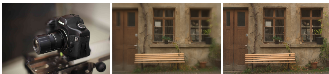
Figure 6.1: Self-made photographic lens with a 120mm focal length. Taken image without and with lens correction.
