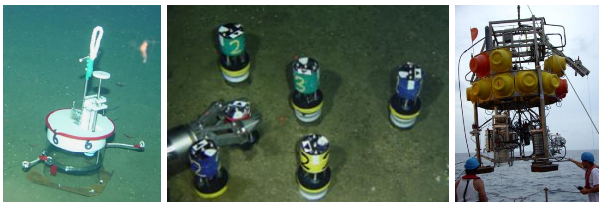
Figure 9 Devices used in the deep sea to perform in-situ feeding experiments: the Oceanlab spreader system (left), incubation or culturing cores (middle), and benthic chamber lander (right). Pictures are property of JAMSTEC (left, middle) and MBARI (right).
