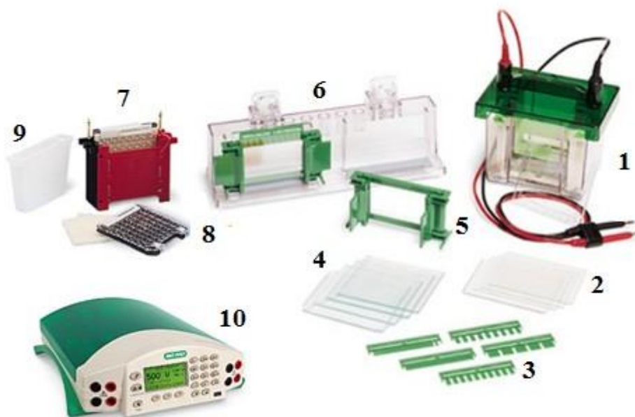
Figure 15. Western blotting equipment. 1-Buffer tank lid with electrode assembly, 2-Membrane, 3-Comb, 4-Glasses 5-Casting Frame, 6-Casting stand 7-Electrode assembly, 8-Gel holder cassette and foam pads 9- Ice cooling unit 10-power supply.
