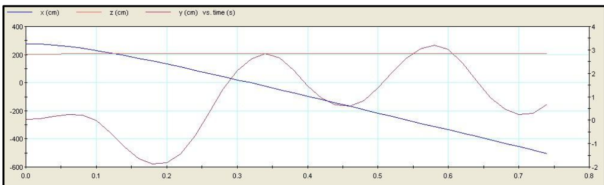
Figure 205: The diagram displays the position of the center of mass along the y-axis during the bipedal gait E simulation with octuple velocity and arms directed straight back.
