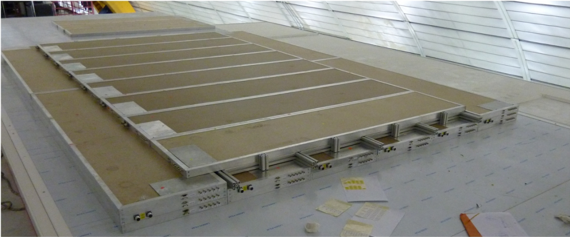
Figure 5.6: An image of the scintillator panel veto on top of the GERDA clean room.
