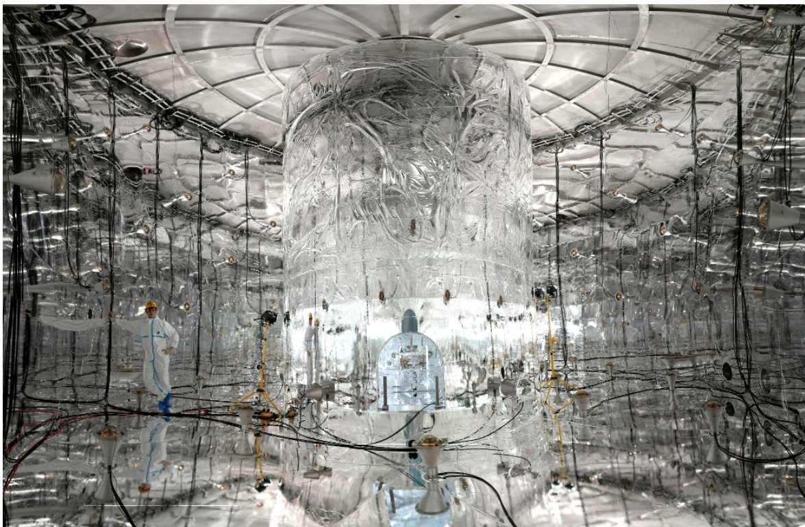
Figure 5.2: A view inside the Cherenkov water veto. The inner walls of the water tank, the outer walls of the cryostat, the pillbox and the floor plate are covered with reflective foil. Several mounted PMTs can be seen.
