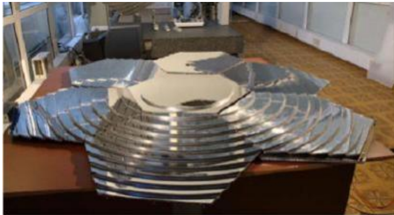
Figure 3.8.2: Segmented Fresnel mirror of the TUS detector. Taken from [93].
