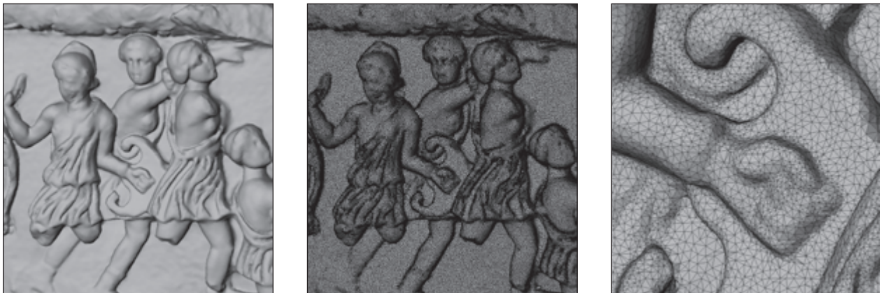
Figure 4. Left: Scan data captured with structured light scanner; Middle: triangular meshing; Right: detail area (© Breuckmann).
