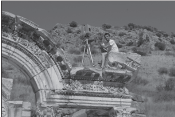
Figure 5. Left: 3D Scanning with Z+F laser scanner; Right: Point cloud from 3D laser scans (© ÖAI).
