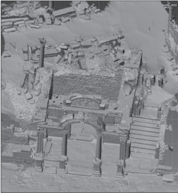
Figure 7. Combination of structured light scan data and laser scan data (© Breuckmann).
