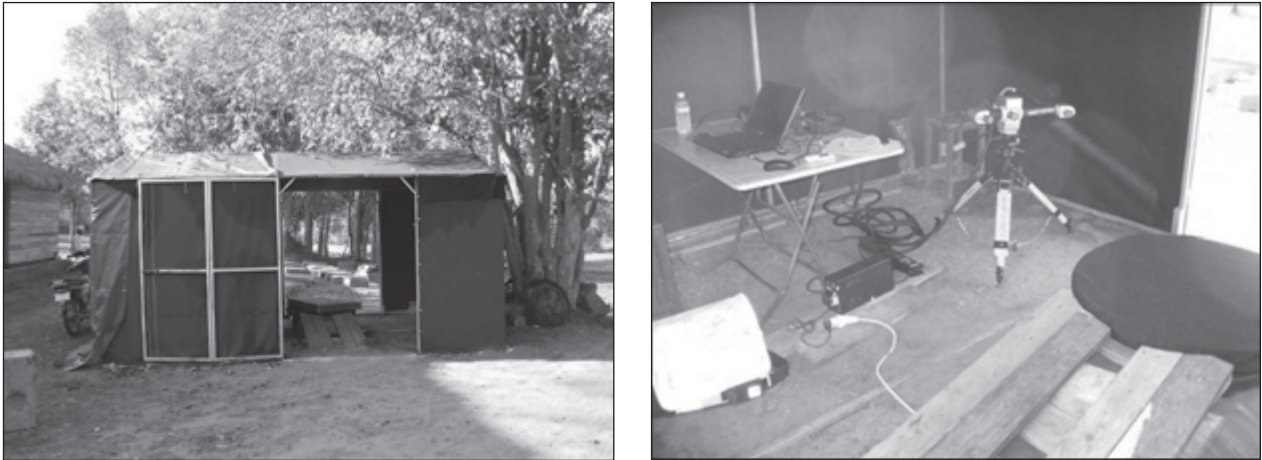
Figure 4. Setup of the 3D scanner for acquisition of the stones in (a) the tent with (b) the turn table and the ramp. Picture Source: Dr. Pheakdey Nguonphan.
