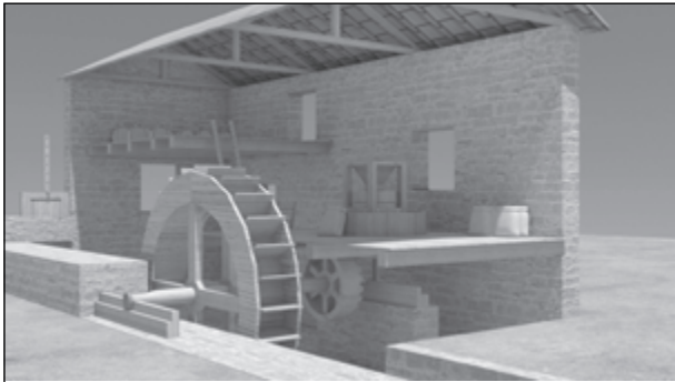
Figure 2. Vitruvius's water mill (1 st century BC).
