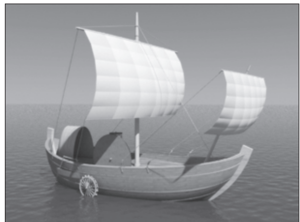
Figure 3. Vitruvius's maritime odometer (1 st century BC).
