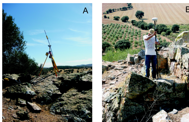
Figure 5: DGPS in the field. A.-Base station placed in a fixed point tied to the National Geodetic Network. B.-Measuring with the rover pole.
