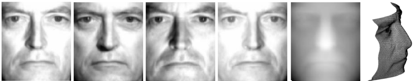
Figure 5: Six images (4 of which are shown) of the face of one of the co-author, D. Mumford, are used to determine its shape. The pose is constant, while the lighting varies. The resulting photometric variation reveals the shape, as shown in the depth map and wire-frame (fifth and sixth pictures).
